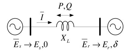
Active/reactive power at sending end | Active/reactive power at receiving  $E_{s}$
