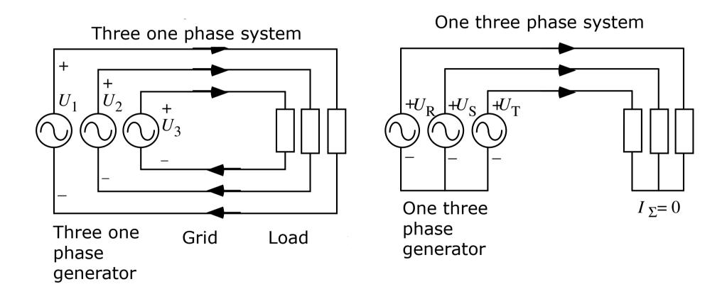
The lowest number of phases that could create a rotating electric field
