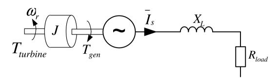
$$J\frac{d\omega_{r}}{dt} = T_{turbine} - T_{gen}$$
