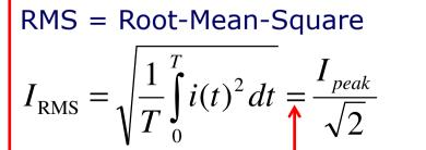
Only for sinusoidal waveforms
